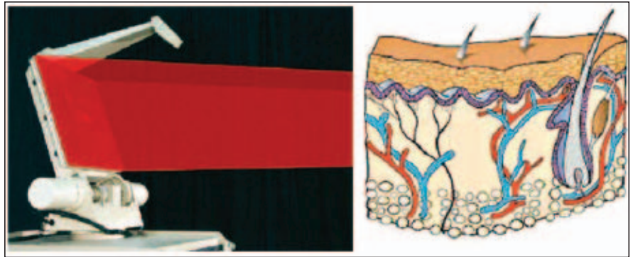
▲ Fig. 6 Silent Guardian emits a focused beam that heats the water molecules around the skin's pain and heat receptors, creating a burning sensation intended to get the aggressor's attention and repel them.
